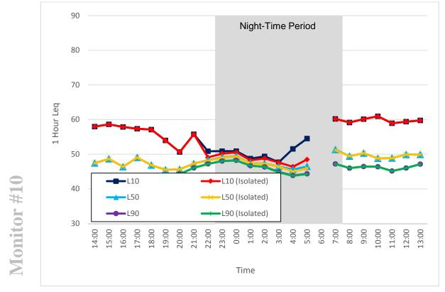
Figure 82. Noise Monitor #10, 1-Hour L<sub>10</sub>, L<sub>50</sub>, L<sub>90</sub> L<sub>eq</sub> Sound Levels (August 20 - 21, 2014)<sup>1</sup>
