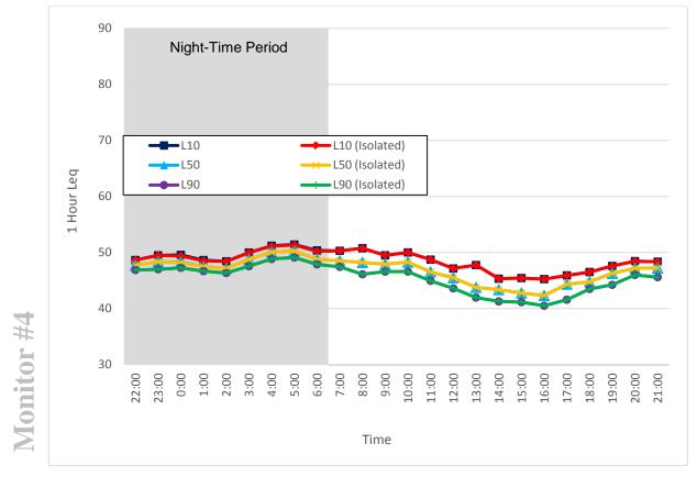
Figure 42. Noise Monitor #4, 1-Hour L<sub>10</sub>, L<sub>50</sub>, L<sub>90</sub> L<sub>eq</sub> Sound Levels (June 16 - 17, 2014)
