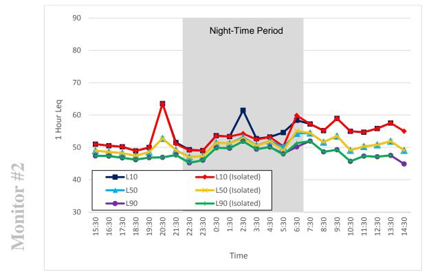
Figure 26. Noise Monitor #2, 1-Hour L<sub>10</sub>, L<sub>50</sub>, L<sub>90</sub> L<sub>eq</sub> Sound Levels (August 13 - 14, 2014)
