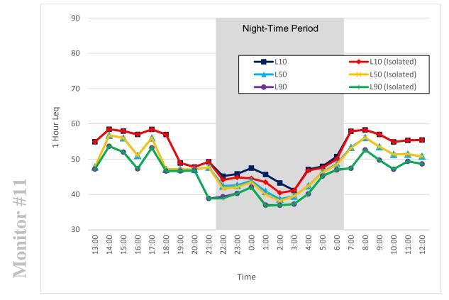
Figure 90. Noise Monitor #11, 1-Hour L<sub>10</sub>, L<sub>50</sub>, L<sub>90</sub> L<sub>eq</sub> Sound Levels (August 13 - 14, 2014)
