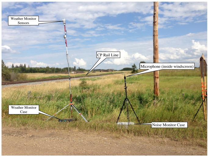
Figure 13. Noise Monitor #12 (With Weather Monitor)
