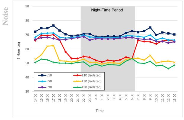
Figure 19. Noise Monitor #1, 1-Hour L<sub>10</sub>, L<sub>50</sub>, L<sub>90</sub> L<sub>eq</sub> Sound Levels (August 21 - 22, 2014)
