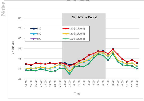
Figure 59. Noise Monitor #6, 1-Hour L<sub>10</sub>, L<sub>50</sub>, L<sub>90</sub> L<sub>eq</sub> Sound Levels (August 14 - 15, 2014)
