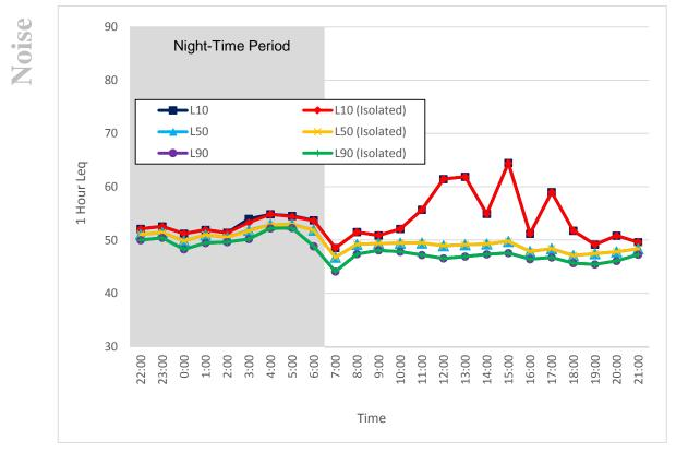
Figure 43. Noise Monitor #4, 1-Hour L<sub>10</sub>, L<sub>50</sub>, L<sub>90</sub> L<sub>eq</sub> Sound Levels (June 25 - 26, 2014)
