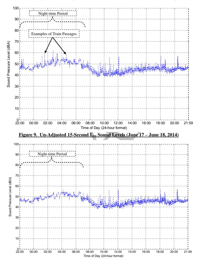
Figure 10. Isolated 15-Second Leg Sound Levels (June 17 – June 18, 2014)
