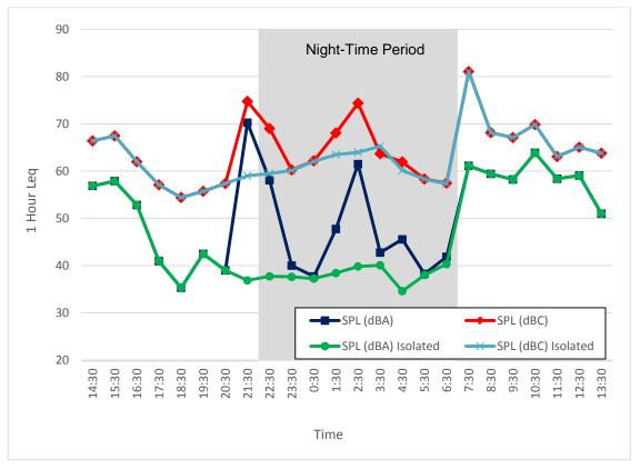
Figure 96. Noise Monitor #12, 1-Hour Leg Sound Levels (August 13 - 14, 2014)
