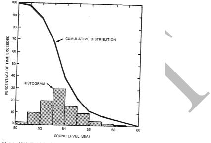
Figure 16.6 Statistically processed community noise showing histogram and cumulative distribution of A weighted sound levels.
