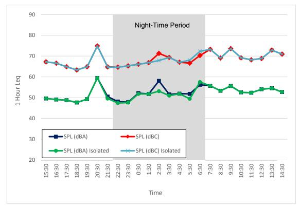
Figure 24. Noise Monitor #2, 1-Hour Leg Sound Levels (August 13 - 14, 2014)
