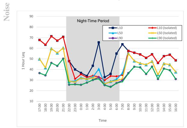
Figure 106. Noise Monitor #12, 1-Hour L<sub>10</sub>, L<sub>50</sub>, L<sub>90</sub> L<sub>eq</sub> Sound Levels (August 21 - 22, 2014)
