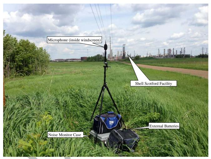
Figure 2. Noise Monitor Used for Environmental Noise Study
