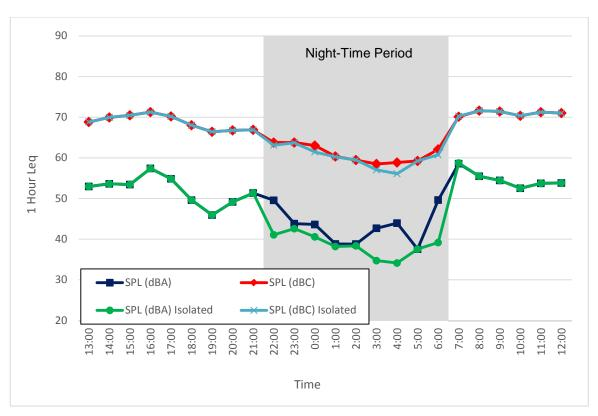
Figure 89. Noise Monitor #11, 1-Hour Leg Sound Levels (August 14 - 15, 2014)
