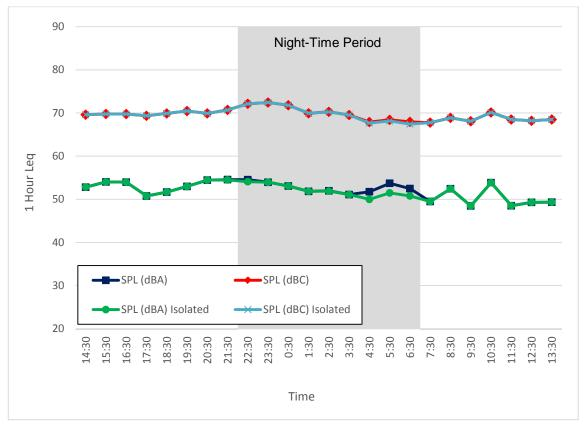
Figure 48. Noise Monitor #5, 1-Hour Leg Sound Levels (August 13 - 14, 2014)
