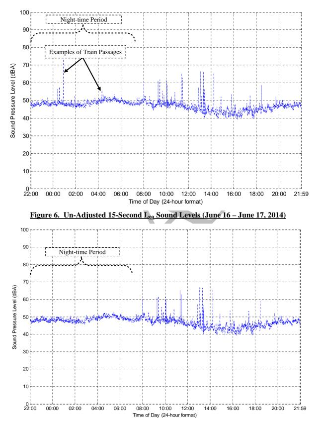
Figure 7. Isolated 15-Second Leg Sound Levels (June 16 – June 17, 2014)
