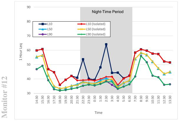
Figure 98. Noise Monitor #12, 1-Hour L<sub>10</sub>, L<sub>50</sub>, L<sub>90</sub> L<sub>eq</sub> Sound Levels (August 13 - 14, 2014)
