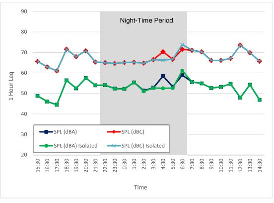
Figure 25. Noise Monitor #2, 1-Hour Leg Sound Levels (August 14 - 15, 2014)
