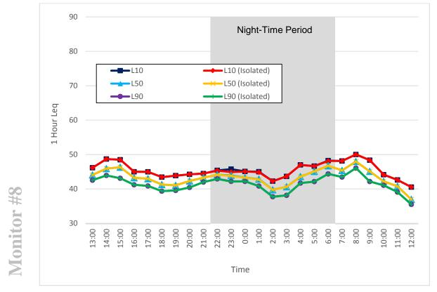
Figure 66. Noise Monitor #8, 1-Hour L<sub>10</sub>, L<sub>50</sub>, L<sub>90</sub> L<sub>eq</sub> Sound Levels (August 13 - 14, 2014)
