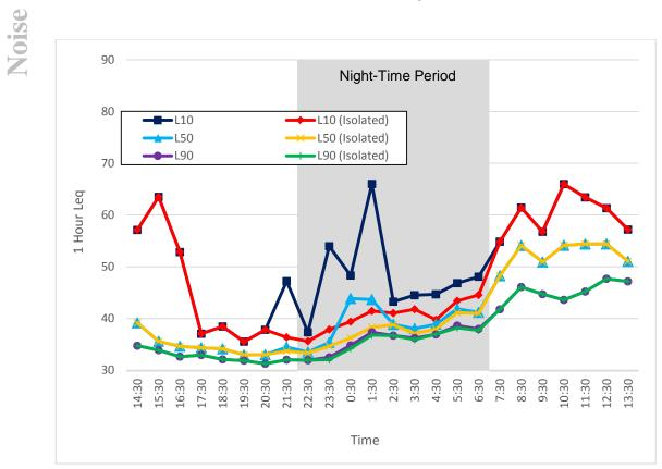
Figure 99. Noise Monitor #12, 1-Hour L<sub>10</sub>, L<sub>50</sub>, L<sub>90</sub> L<sub>eq</sub> Sound Levels (August 14 - 15, 2014)
