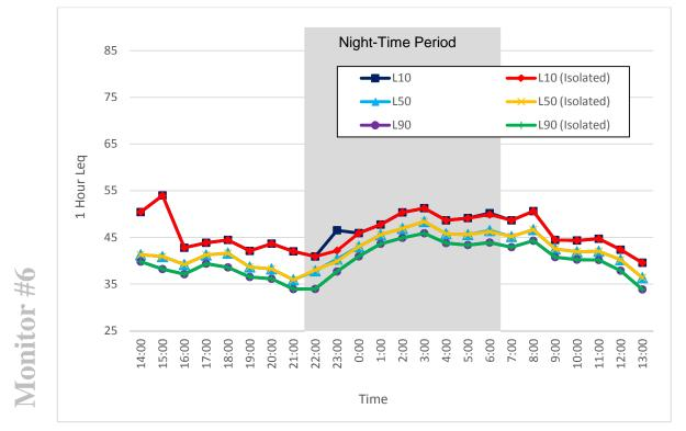
Figure 58. Noise Monitor #6, 1-Hour L<sub>10</sub>, L<sub>50</sub>, L<sub>90</sub> L<sub>eq</sub> Sound Levels (August 13 - 14, 2014)
