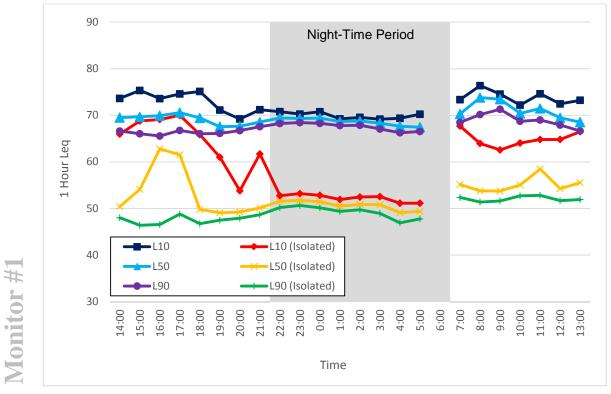
Figure 18. Noise Monitor #1, 1-Hour L<sub>10</sub>, L<sub>50</sub>, L<sub>90</sub> L<sub>eq</sub> Sound Levels (August 20 - 21, 2014)<sup>1</sup>
