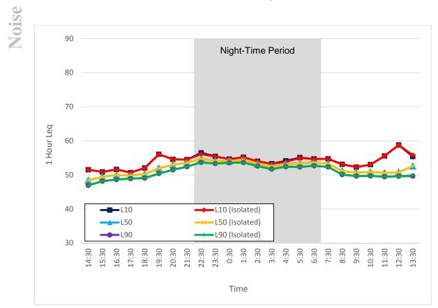
Figure 51. Noise Monitor #5, 1-Hour L<sub>10</sub>, L<sub>50</sub>, L<sub>90</sub> L<sub>eq</sub> Sound Levels (August 14 - 15, 2014)
