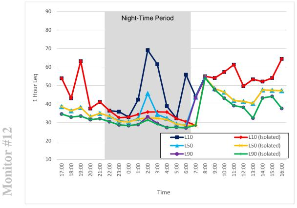
Figure 105. Noise Monitor #12, 1-Hour L<sub>10</sub>, L<sub>50</sub>, L<sub>90</sub> L<sub>eq</sub> Sound Levels (August 20 - 21, 2014)
