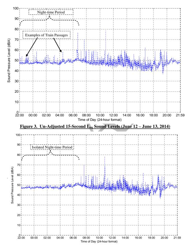
Figure 4. Isolated 15-Second Leg Sound Levels (June 12 – June 13, 2014)
