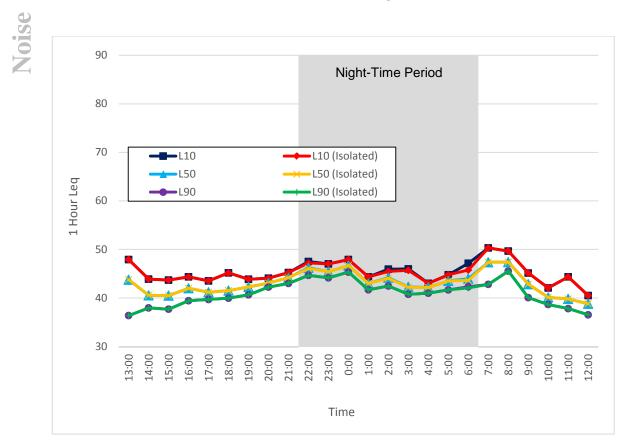
Figure 67. Noise Monitor #8, 1-Hour L<sub>10</sub>, L<sub>50</sub>, L<sub>90</sub> L<sub>eq</sub> Sound Levels (August 14 - 15, 2014)
