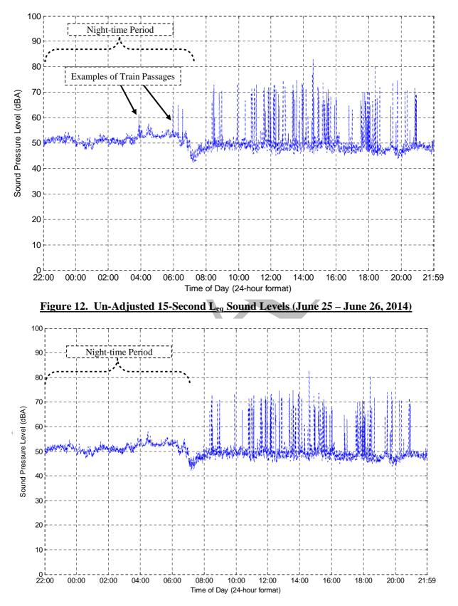
Figure 13. Isolated 15-Second Leg Sound Levels (June 25 – June 26, 2014)
