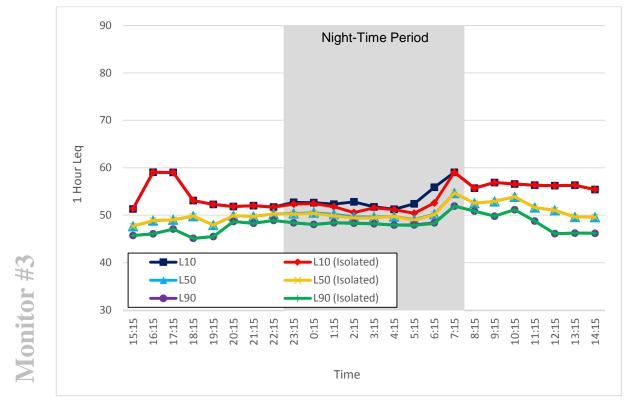
Figure 34. Noise Monitor #3, 1-Hour L<sub>10</sub>, L<sub>50</sub>, L<sub>90</sub> L<sub>eq</sub> Sound Levels (August 13 - 14, 2014)
