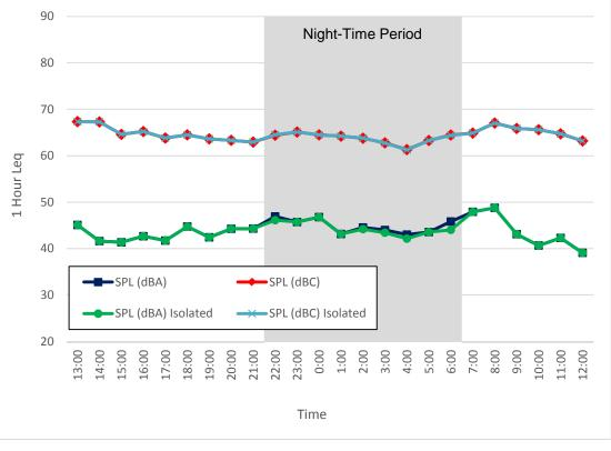
Figure 65. Noise Monitor #8, 1-Hour Leg Sound Levels (August 14 - 15, 2014)
