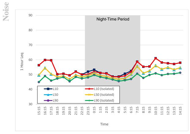
Figure 35. Noise Monitor #3, 1-Hour L<sub>10</sub>, L<sub>50</sub>, L<sub>90</sub> L<sub>eq</sub> Sound Levels (August 14 - 15, 2014)
