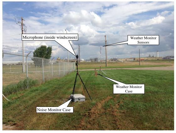
Figure 11. Noise Monitor #10 (With Weather Monitor)
