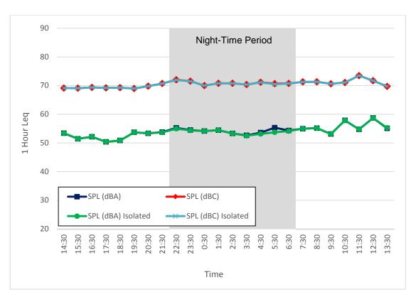
Figure 49. Noise Monitor #5, 1-Hour Leg Sound Levels (August 14 - 15, 2014)
