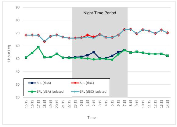
Figure 32. Noise Monitor #3, 1-Hour Leg Sound Levels (August 13 - 14, 2014)
