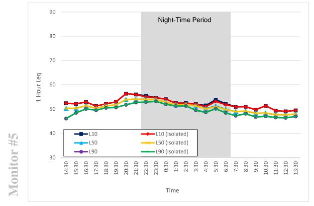
Figure 50. Noise Monitor #5, 1-Hour L<sub>10</sub>, L<sub>50</sub>, L<sub>90</sub> L<sub>eq</sub> Sound Levels (August 13 - 14, 2014)
