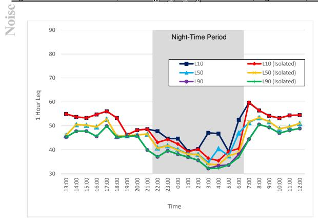
Figure 91. Noise Monitor #11, 1-Hour L<sub>10</sub>, L<sub>50</sub>, L<sub>90</sub> L<sub>eq</sub> Sound Levels (August 14 - 15, 2014)
